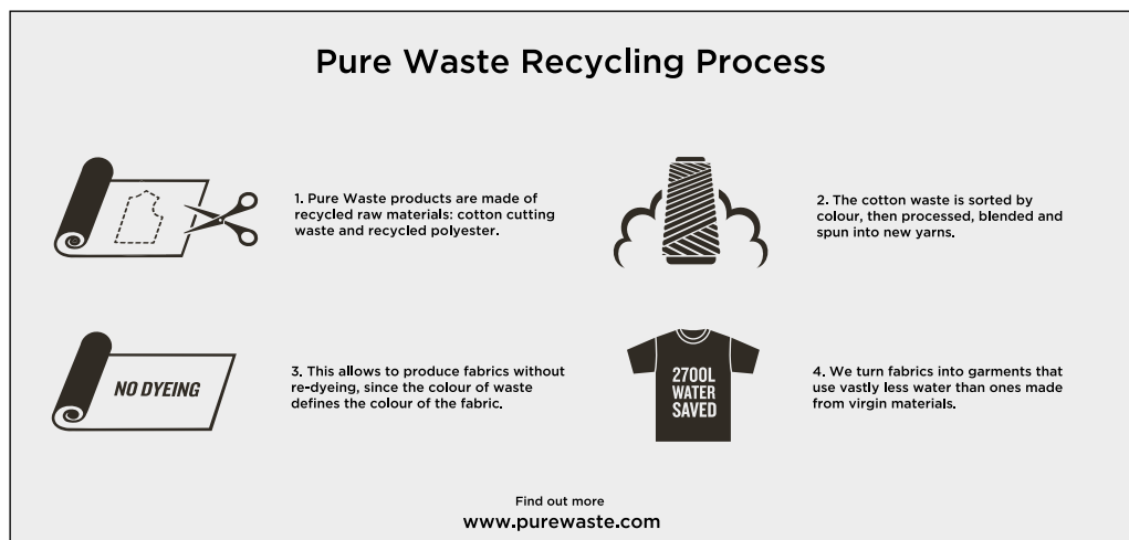
Figure 20. Mechanical recycling used by Pure Waste 60
