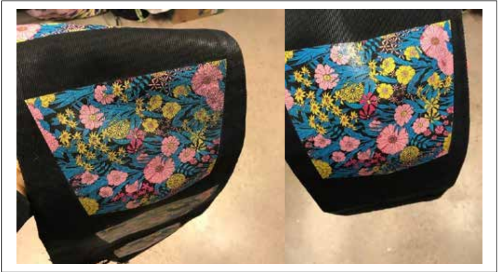
Figure 7. Example of print pilot testing with different amounts of pre-treatment applied to a jeans pocket (Ertelt, Guzun & Scott 2018).
